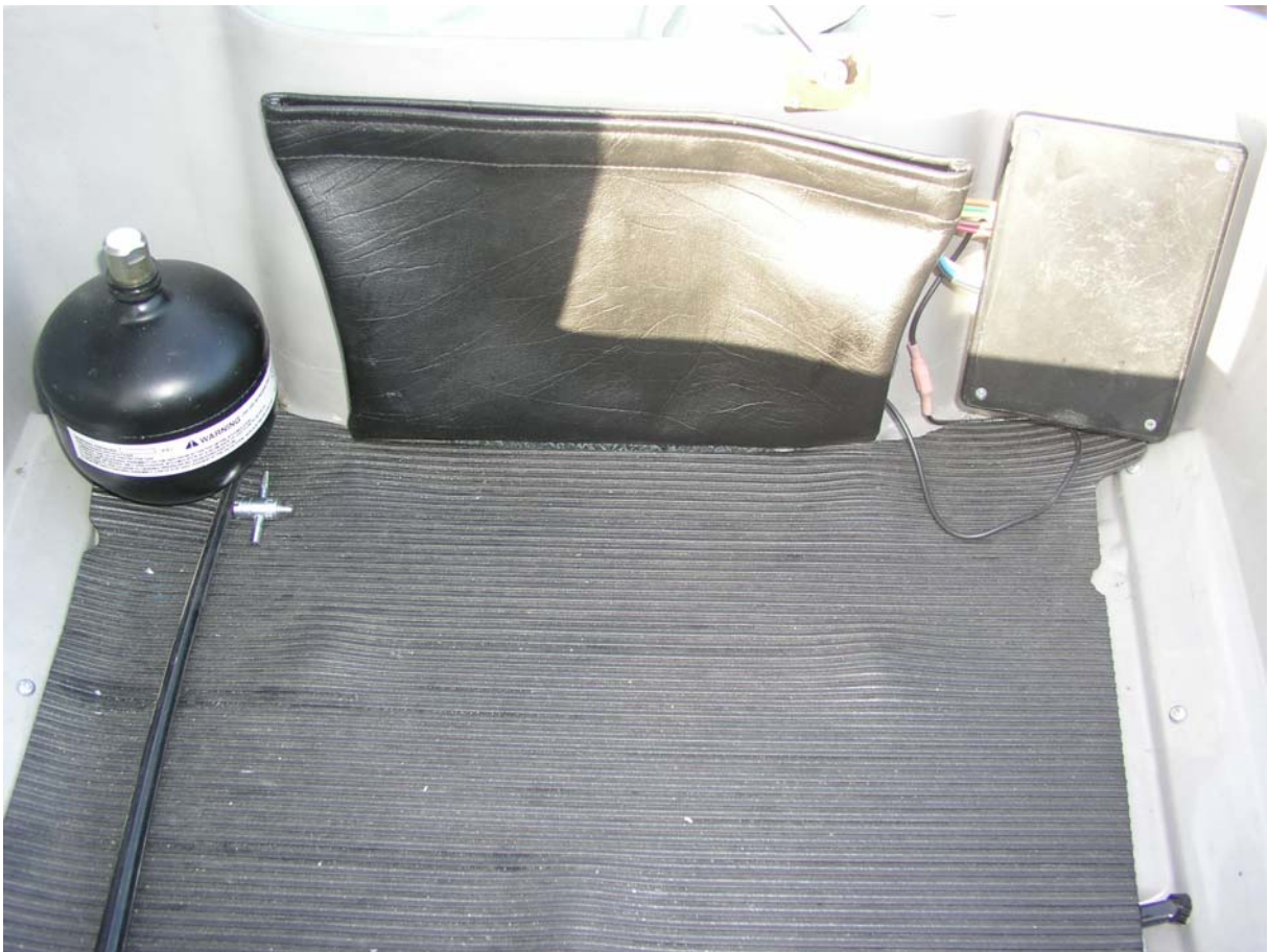
Accumulator Tank mounted in trunk. See appendix for a picture of a saddle bag installation.
