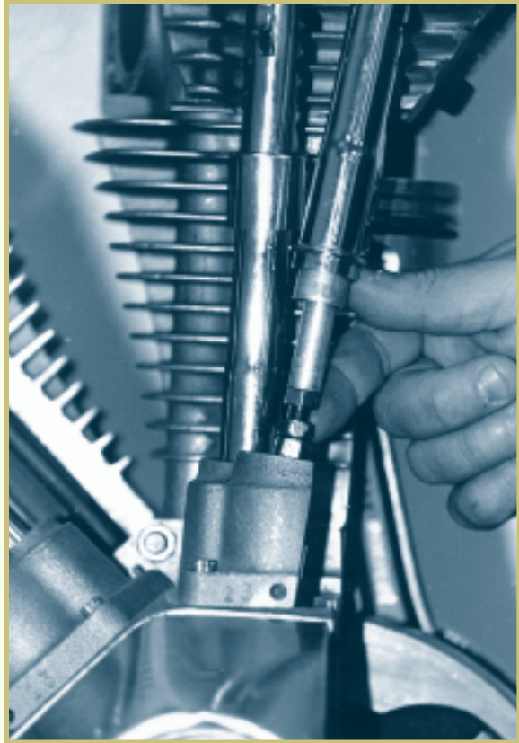
FIGURE 14—The push rod has an adjuster built into it for finer adjustments to the hydraulic-valve lifter system.
