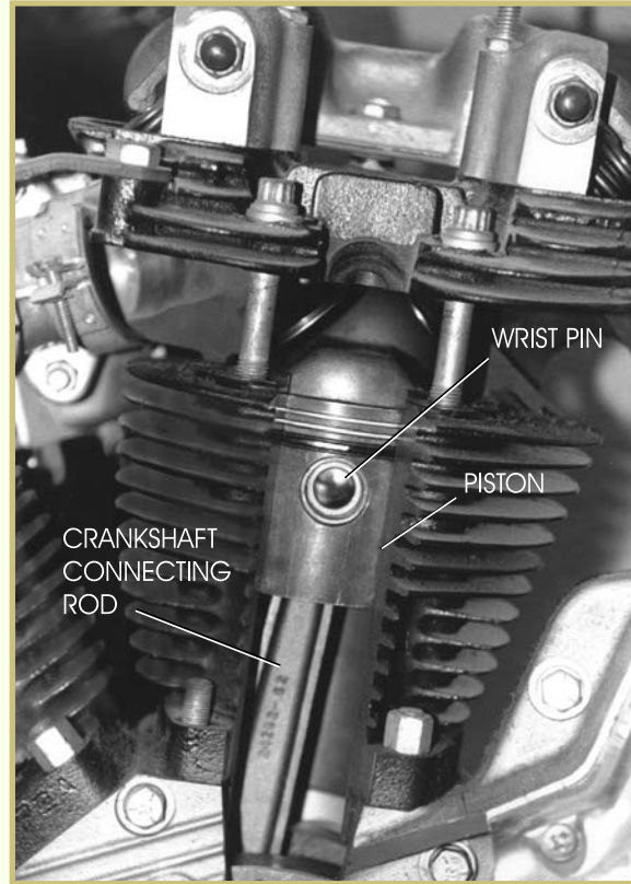
FIGURE 16 —The piston is shown attached to the crankshaft connecting rod.
