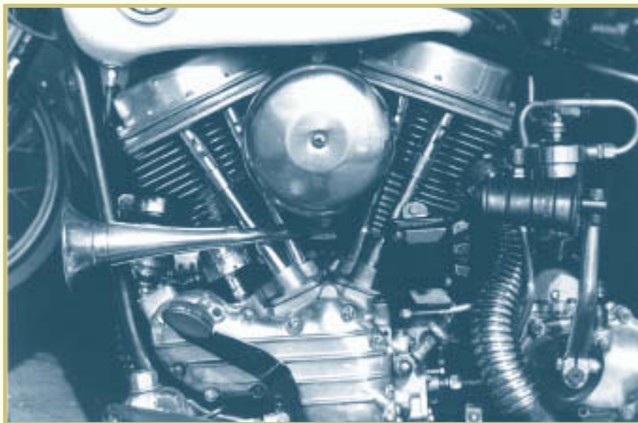
FIGURE 3 —The Panhead engine superseded the Knucklehead engine because of its light weight, power, and better oiling system.
