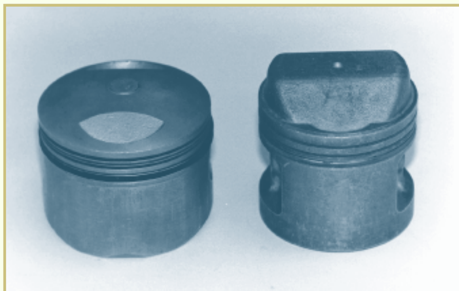
FIGURE 12 —Two different V-twin pistons are shown here. The pistons have pockets machined into them to prevent contact with the valves.
